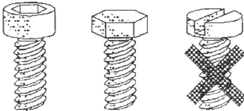
Allen Screws / Hexagon Screw / Slotted Screw
